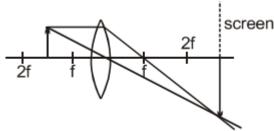
If the whole set up is immersed in water without disturbing the object and the screen positions, what will one observe on the screen?
